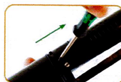
Use the small hole at the bottom of the sensor to lever the sensor out.
