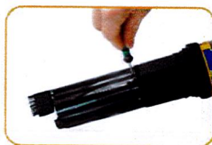
Use included hex wrench to loosen set screw on RDO sensor.
