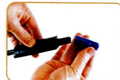
Remove the dust cover from the RDO sensor.
